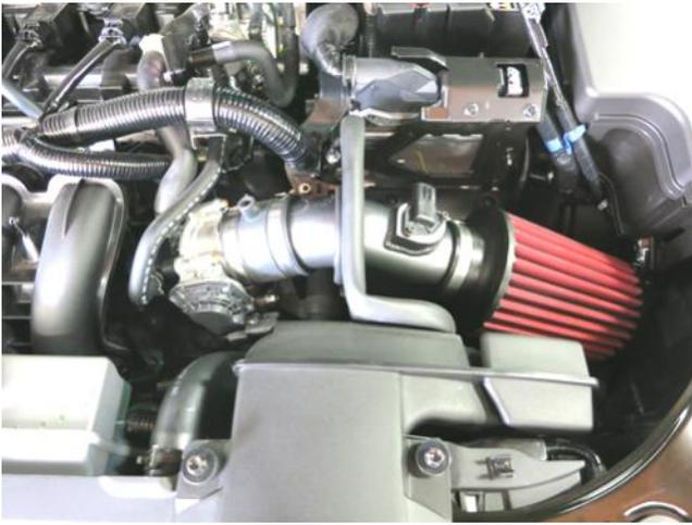
k. Carefully install intake tube and install provided 16" edge trim around top edge of heat shield as shown.
